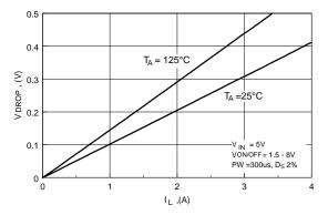
Figure 1. Conduction Voltage Drop
