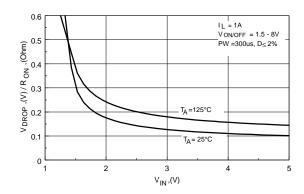
Figure 4. On-Resistance Variation with Input Voltage.
