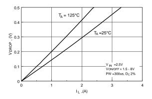
Figure 3. Conduction Voltage Drop Variation with Load Current.
