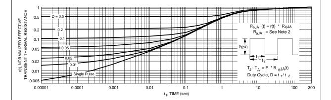
Figure 5. Transient Thermal Response Curve.
