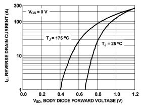
Figure 8. Forward Diode Characteristics
