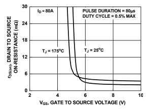
Figure 11. Rdson vs Gate Voltage
