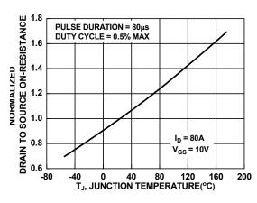
Figure 12. Normalized Rdson vs Junction Temperature
