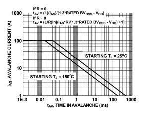
Figure 6. Unclamped Inductive Switching Capability
