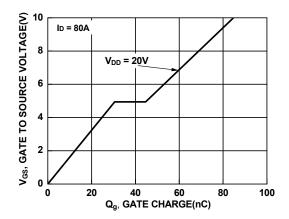
Figure 16. Gate Charge vs Gate to Source Voltage
