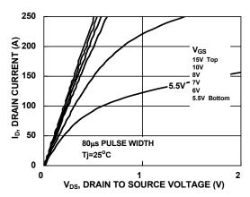
Figure 9. Saturation Characteristics
