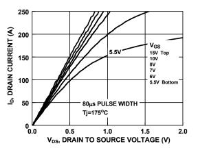
Figure 10. Saturation Characteristics
