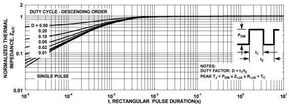
Figure 3. Normalized Maximum Transient Thermal Impedance
