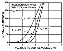
Figure 7. Transfer Characteristics
