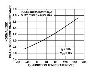
Figure 12. Normalized R<sub>DSON</sub> vs. Junction Temperature
