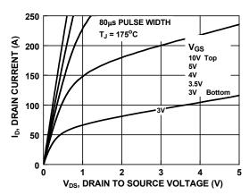
Figure 10. Saturation Characteristics
