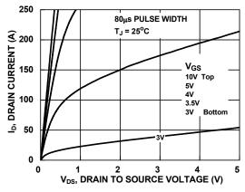
Figure 9. Saturation Characteristics
