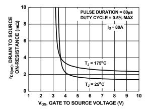
Figure 11. R<sub>DSON</sub> vs. Gate Voltage
