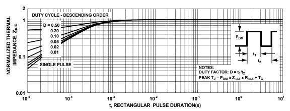
Figure 3. Normalized Maximum Transient Thermal Impedance
