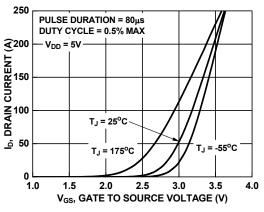
Figure 7. Transfer Characteristics
