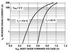
Figure 8. Forward Diode Characteristics
