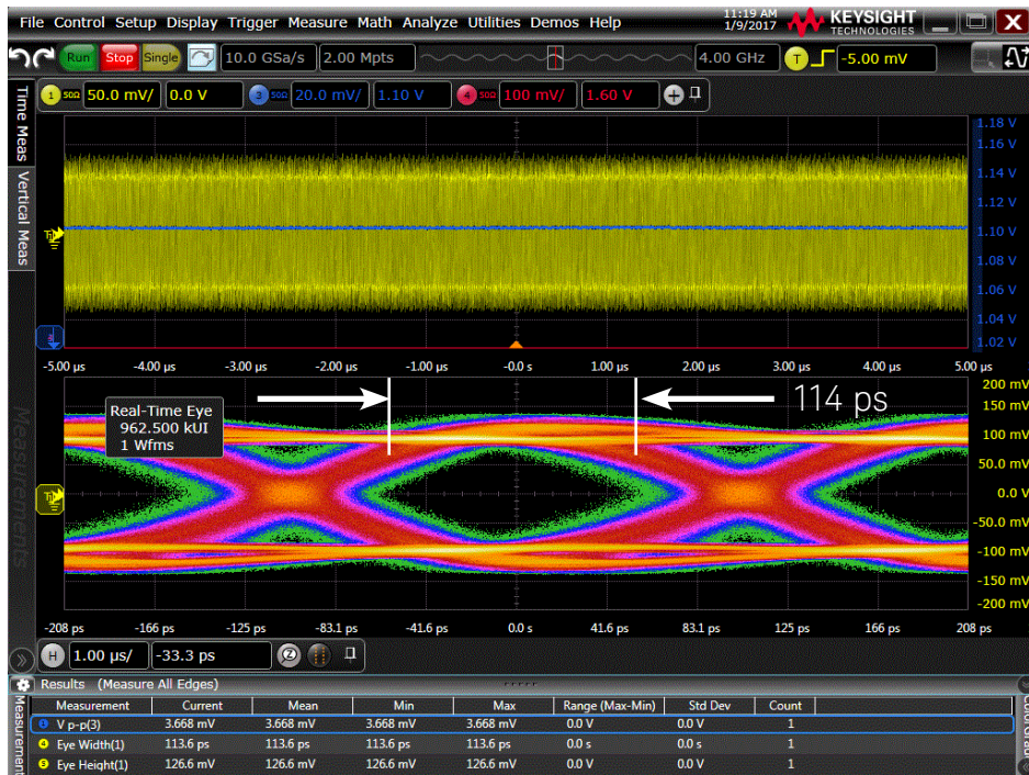
Figure 25. Eye diagram of FPGA serial data after the DC supply was cleaned-up. Notice the increased width of the eye.
