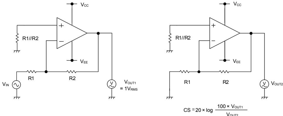
Figure 62. Test Circuit 3 (Channel Separation)
