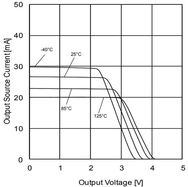
Figure 35. Output Source Current vs Output Voltage ( $V_{CC}=5V$ )
