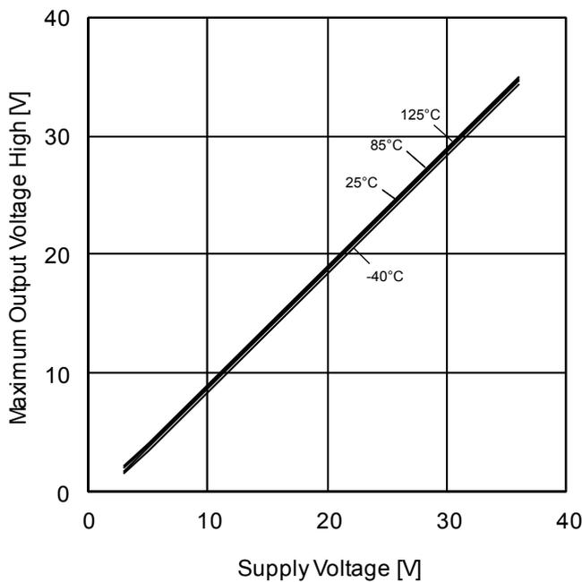
Figure 3. Maximum Output Voltage (High) vs Supply Voltage (R<sub>L</sub>=10kΩ)
