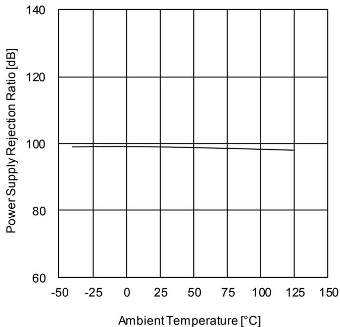
Figure 29. Power Supply Rejection Ratio vs Ambient Temperature
