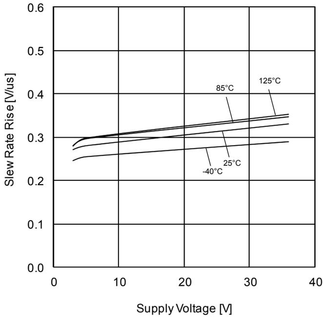
Figure 50. Slew Rate Rise vs Supply Voltage
