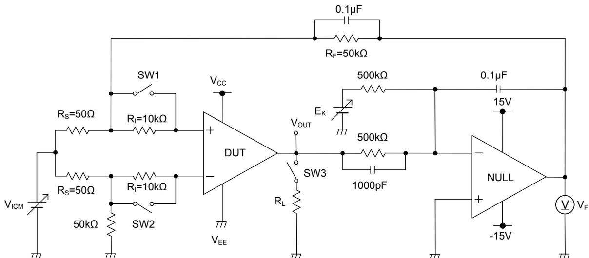
Figure 59. Test Circuit 1 (One Channel Only)
