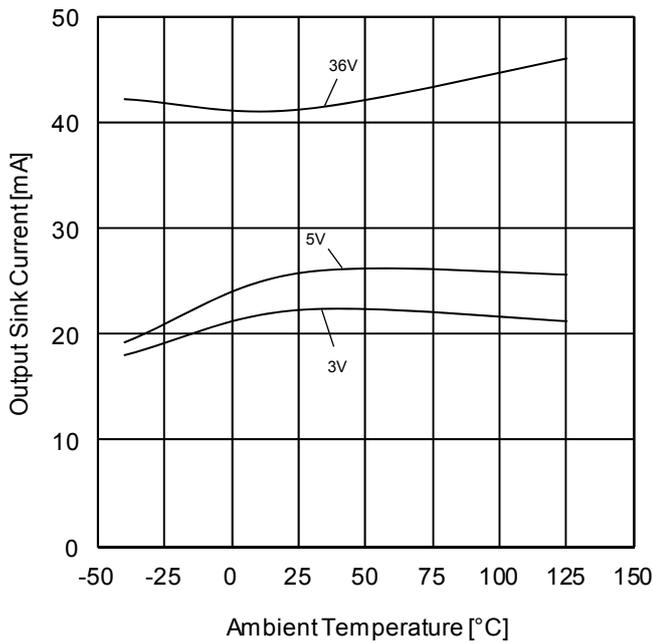
Figure 38. Output Sink Current vs Ambient Temperature ( $V_{OUT}=V_{CC}$ )
