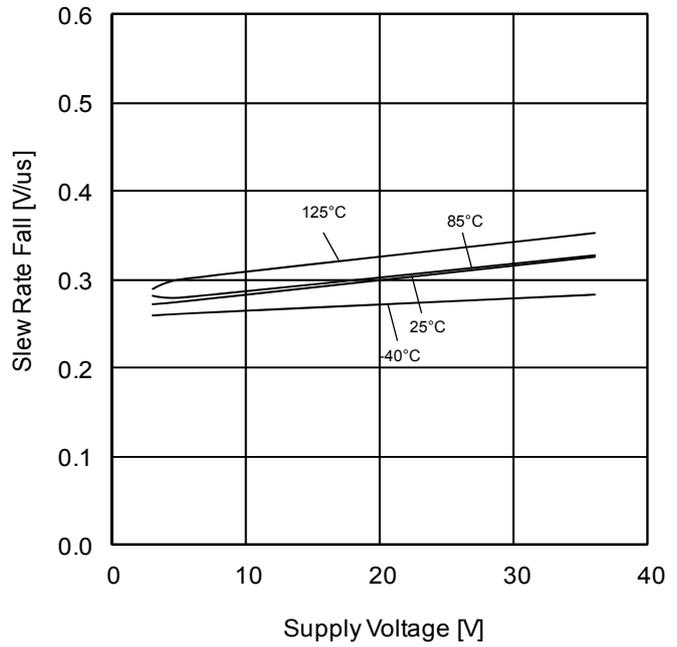
Figure 51. Slew Rate Fall vs Supply Voltage
