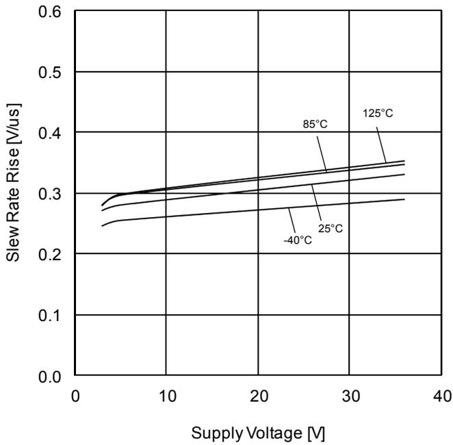
Figure 21. Slew Rate Rise vs Supply Voltage
