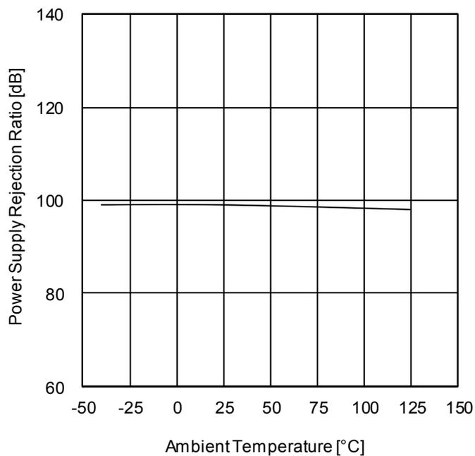
Figure 58. Power Supply Rejection Ratio vs Ambient Temperature
