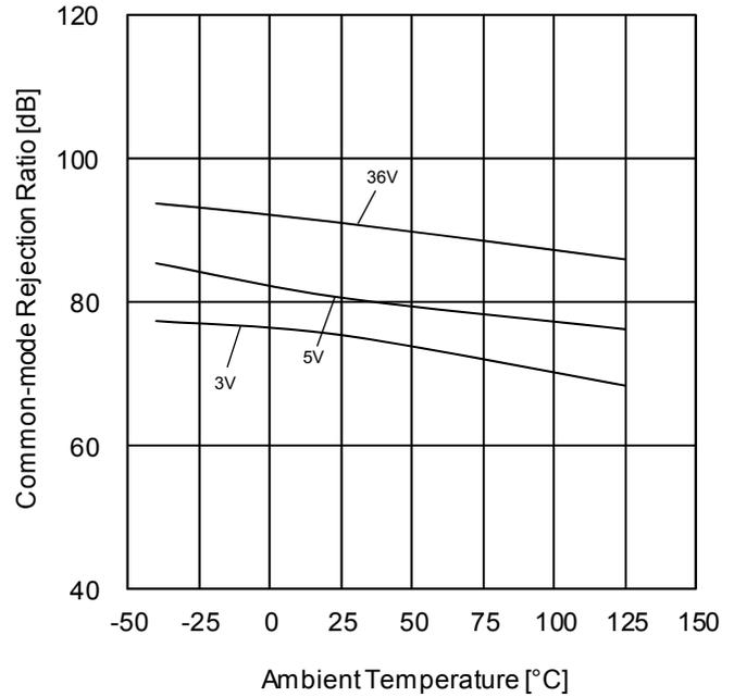
Figure 57. Common-mode Rejection Ratio vs Ambient Temperature
