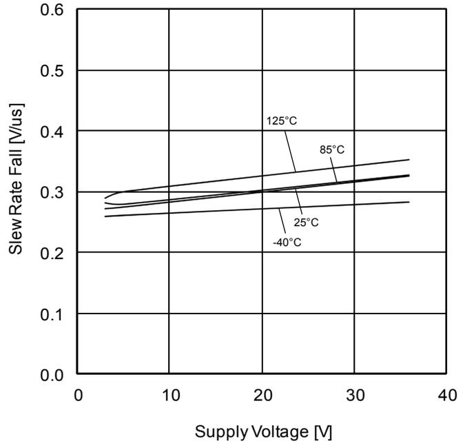
Figure 22. Slew Rate Fall vs Supply Voltage
