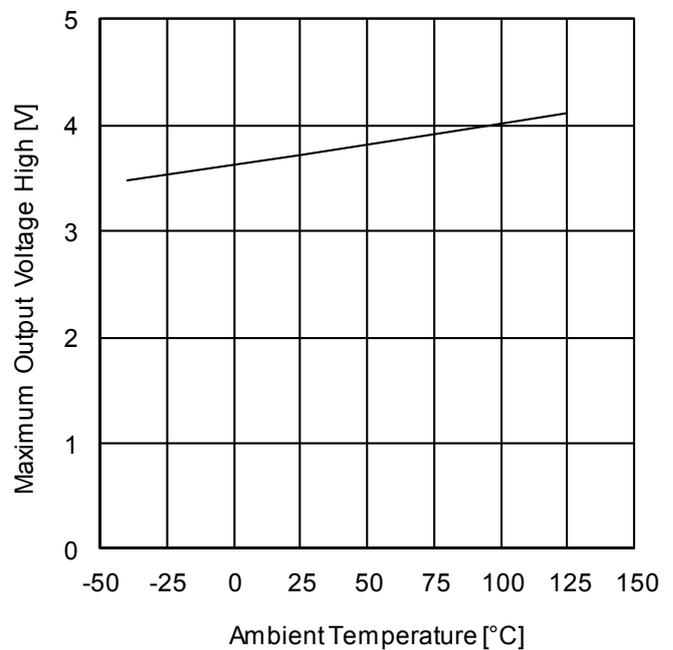
Figure 4. Maximum Output Voltage (High) vs Ambient Temperature (V<sub>CC</sub>=5V, R<sub>L</sub>=10kΩ)
