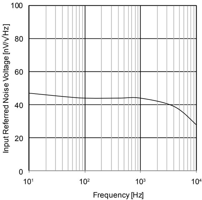
Figure 23. Input Referred Noise Voltage vs Frequency (V<sub>CC</sub>=5V)
