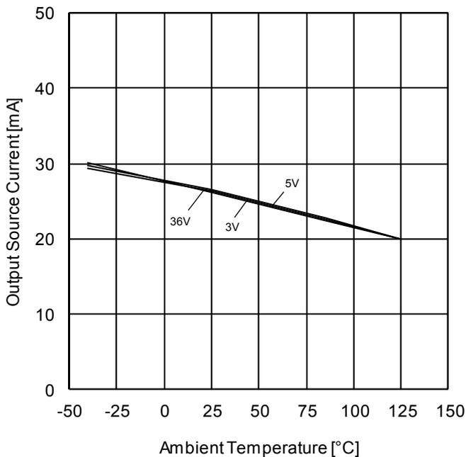
Figure 36. Output Source Current vs Ambient Temperature ( $V_{OUT}=0V$ )
