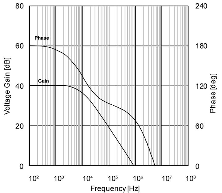
Figure 53. Voltage Gain, Phase vs Frequency
