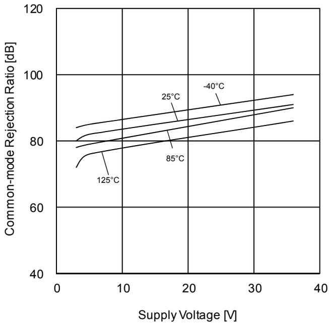
Figure 56. Common-mode Rejection Ratio vs Supply Voltage
