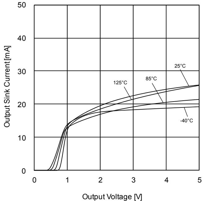
Figure 37. Output Sink Current vs Output Voltage ( $V_{CC}=5V$ )
