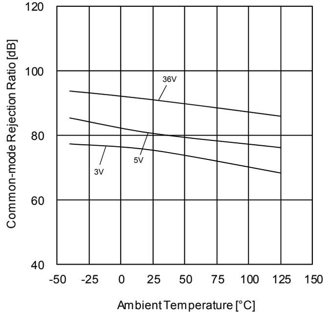
Figure 28. Common-mode Rejection Ratio vs Ambient Temperature
