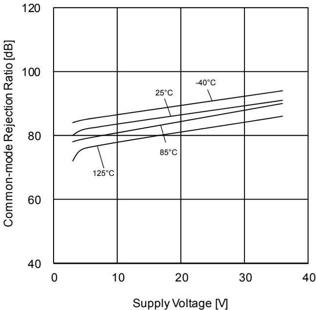
Figure 27. Common-mode Rejection Ratio vs Supply Voltage
