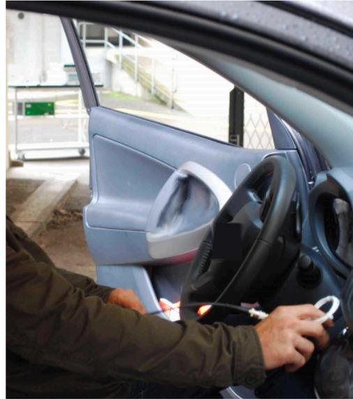
(b) Starting the engine using the relay.
