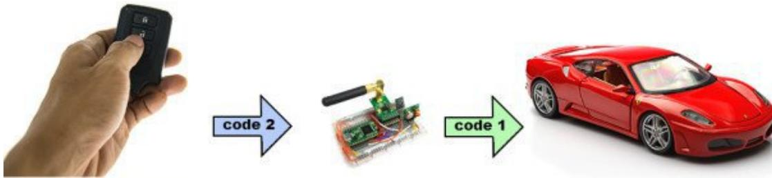
**Figure 10. The user clicks the button again and the RollJam broadcasts the old code while simultaneously capturing the new one. The car unlocks [7].**
