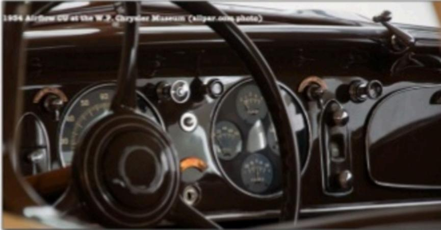
**Figure 1. A car that has no key but two separate buttons – starter and ignition to start the car[2].**
