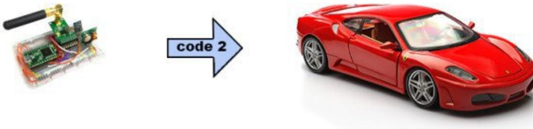
**Figure 11. The RollJam device is retrieved, still holding the new unused code. The code can then be transmitted later to unlock the car [7].**
