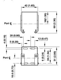
**Neck Mounting** for B72, R72, V72, includes plastic panel nut Use 4 mm (5/32") screws to mount bracket to wall.
