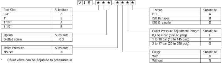
Relief valve can be adjusted to pressures in excess of, and less than, those specified.
