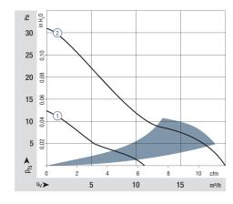
Air performance measured according to: ISO 5801. Installation category A, without contact protection. Noise: Total sound power level  $L_WA$  ISO 103002 measured on a hemisphere with a radius of 2 m. Sound pressure level LpA measured at 1 m distance
