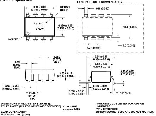
NOTE: FLOATING LEAD PROTRUSION IS 0.25 mm (10 mils) MAX.
