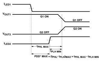
\*PDD = PROPAGATION DELAY DIFFERENCE NOTE: FOR PDD CALCULATIONS THE PROPAGATION DELAYS ARE TAKEN AT THE SAME TEMPERATURE AND TEST CONDITIONS.
