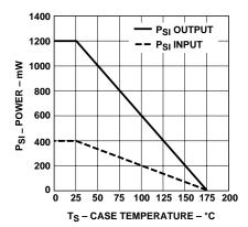
Figure 37b. HCPL-315J: Thermal Derating Curve, Dependence of Safety Limiting Value with Case Temperature per IEC/EN/DIN EN 60747-5-2.
