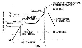
NOTES: THE TIME FROM 25 °C to PEAK TEMPERATURE = 8 MINUTES MAX.  $T_{smax}$  = 200 °C,  $T_{smin}$  = 150 °C
