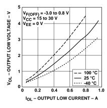
Figure 4.  $\rm V_{OL}$  vs. Temperature.
