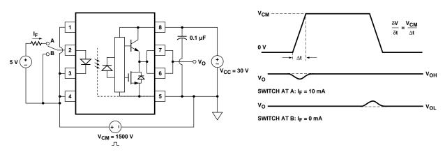
Figure 24. CMR Test Circuit and Waveforms.
