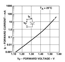
Figure 16. Input Current vs. Forward Voltage.
