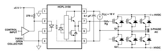
Figure 25a. Recommended LED Drive and Application Circuit.
