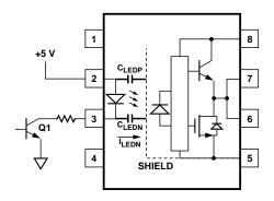
Figure 32. Not Recommended Open Collector Drive Circuit.
