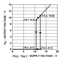
Figure 36. Under Voltage Lock Out.
