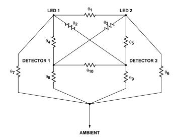
Figure 28b. Thermal Impedance Model for HCPL-315J.
