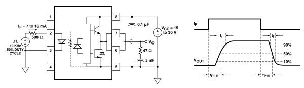
Figure 23. t<sub>PLH</sub>, t<sub>PHL</sub>, t<sub>r</sub>, and t<sub>f</sub> Test Circuit and Waveforms.
