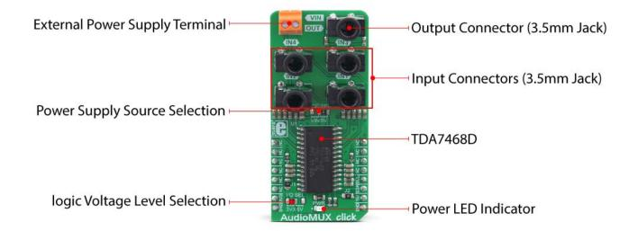
There are four input channels which can be selected over the I2C interface. The IC accepts up to 2.5V peak to peak at its inputs. The impedance of the input terminals is 50 k $\Omega$ , and each input is decoupled by a 440nF capacitor. There are not many registers in this IC, which makes the firmware development very easy. Each channel is routed to a vertically mounted 3.5mm jack, which allows the Click board<sup>TM</sup> to be easily interfaced to an existing audio chain.
