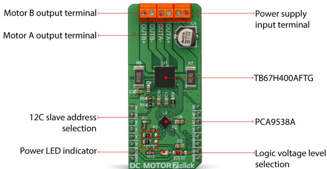
DC MOTOR 7 click requires an external power supply for operation. The optimal voltage that should be used is 24V. Although the TB67H400AFTG driver has both thermal and overcurrent protection, it is just a temporary measure. A short-circuit at the output terminal may damage the Click
