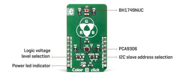
The color intensity sensing is roughly matched to the sensitivity of the human eye, so the sensor is the most sensitive in the range between 500nm and 600nm. The datasheet of the BH1749NUC offers an intensity over the
