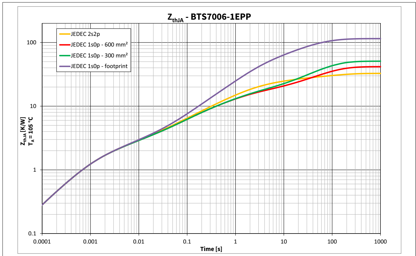
Figure 9 Typical Thermal Impedance. PCB setup according Chapter 4.4.1
