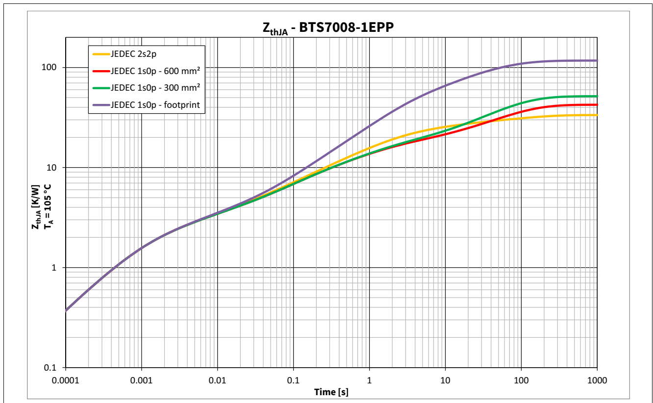
Figure 9 Typical Thermal Impedance. PCB setup according Chapter 4.4.1
