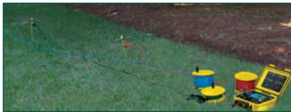
The Model 6472 performs an automated way to measure the value of the earth/ground using the Fall-of-Potential method and storing measurements.
