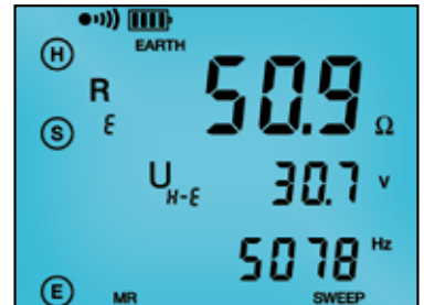
The 3-Point Fall-of-Potential test displaying test lead connection, grounding electrode resistance, test voltage and frequency.
