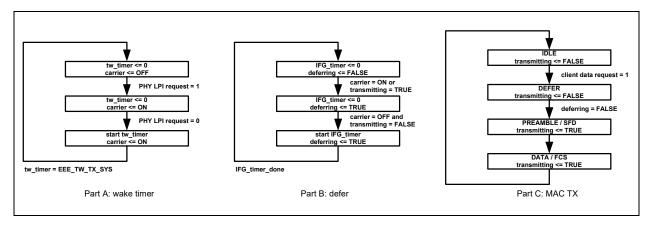
In part A of the figure, a carrier indicator is set when the TX LPI request to the PHY is asserted. The wake timer (tw\_timer) is triggered when the TX LPI request to the PHY is de-asserted and once the wake timer is satisfied, the carrier indicator is cleared. Note that there are separate TX wait values depending on the speed of operation.
