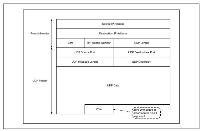
FIGURE 7-10: UDP CHECKSUM - IPV6
