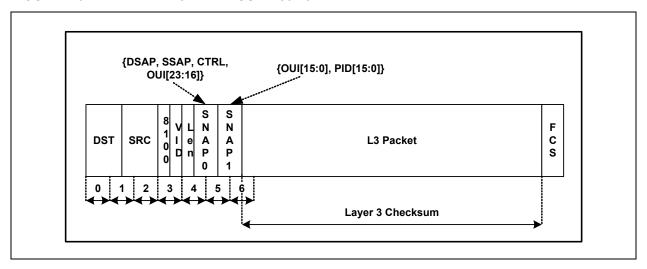
The checksum is placed in the Raw L3 Checksum field in RX Command B. This raw checksum is useful in cases such as when the layer 3 protocol is not IP or IP fragmented packets.
