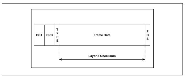
Consider the case where the frame is a 802.3 Ethernet frame with a VLAN tag. The RFE bypasses DA, SA, VLAN tag, SNAP header, and type fields. The calculation begins at the byte immediately following the type field. The calculation does not include the FCS.
