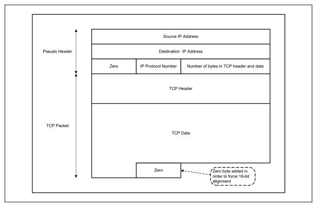
FIGURE 7-8: TCP CHECKSUM - IPV6
