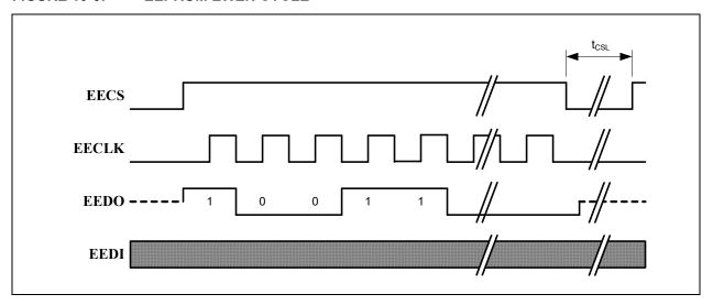
**READ (Read Location):** This command will cause a read of the EEPROM location pointed to by EPC Address (EPC\_ADDR). The result of the read is available in the E2P\_DATA register.
