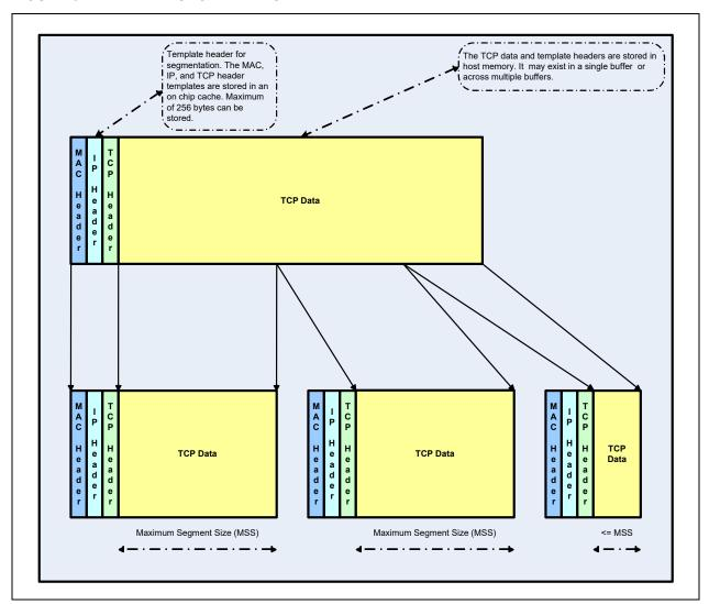
The TCP payload stored in URX buffer RAM is preceded by template headers. They are composed of Ethernet, IP, and TCP headers. The template header may not exceed 256 bytes. The FCT copies the template headers and stores them in the LSO Template Header RAM. They are used as the basis for the headers of all future segments.
