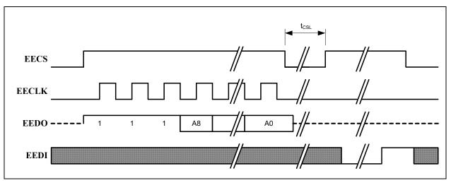
**ERAL (Erase All):** If erase/write operations are enabled in the EEPROM, this command will initiate a bulk erase of the entire EEPROM. The EPC\_TO bit is set if the EEPROM does not respond within 30 ms.
