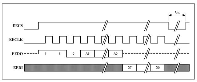
**WRITE (Write Location):** If erase/write operations are enabled in the EEPROM, this command will cause the contents of the E2P\_DATA register to be written to the EEPROM location selected by the EPC Address field (EPC\_ADDR). The EPC\_TO bit is set if the EEPROM does not respond within 30 ms.
