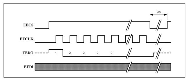
**EWEN (Erase/Write Enable):** Enables the EEPROM for erase and write operations. The EEPROM will allow erase and write operations until the "Erase/Write Disable" command is sent, or until power is cycled.
