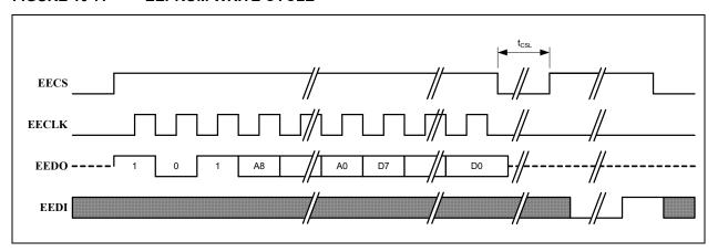
**WRAL (Write All):** If erase/write operations are enabled in the EEPROM, this command will cause the contents of the E2P\_DATA register to be written to every EEPROM memory location. The EPC\_TO bit is set if the EEPROM does not respond within 30 ms.
