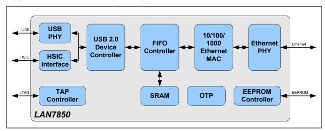
FIGURE 2-1: INTERNAL BLOCK DIAGRAM
