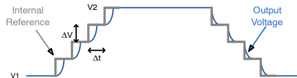
Figure 44. DVS in Forced PPWM Mode Diagram
