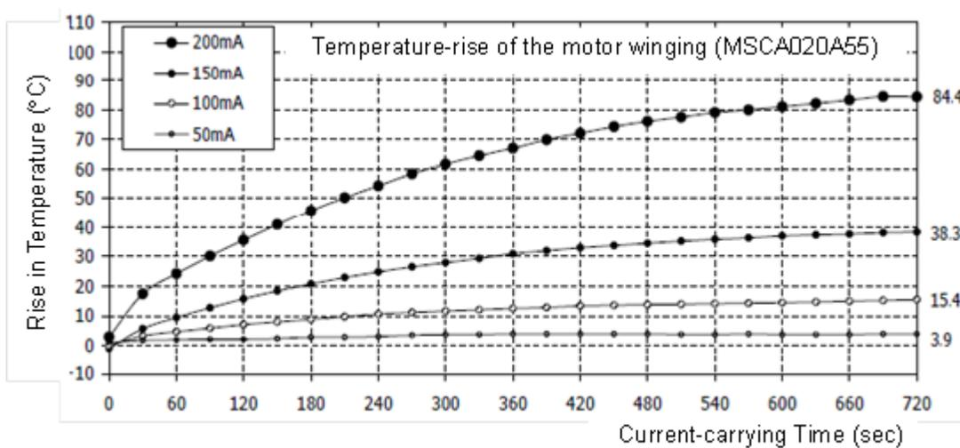
**Figure 6. Temperature-rise characteristic of the motor winding**
