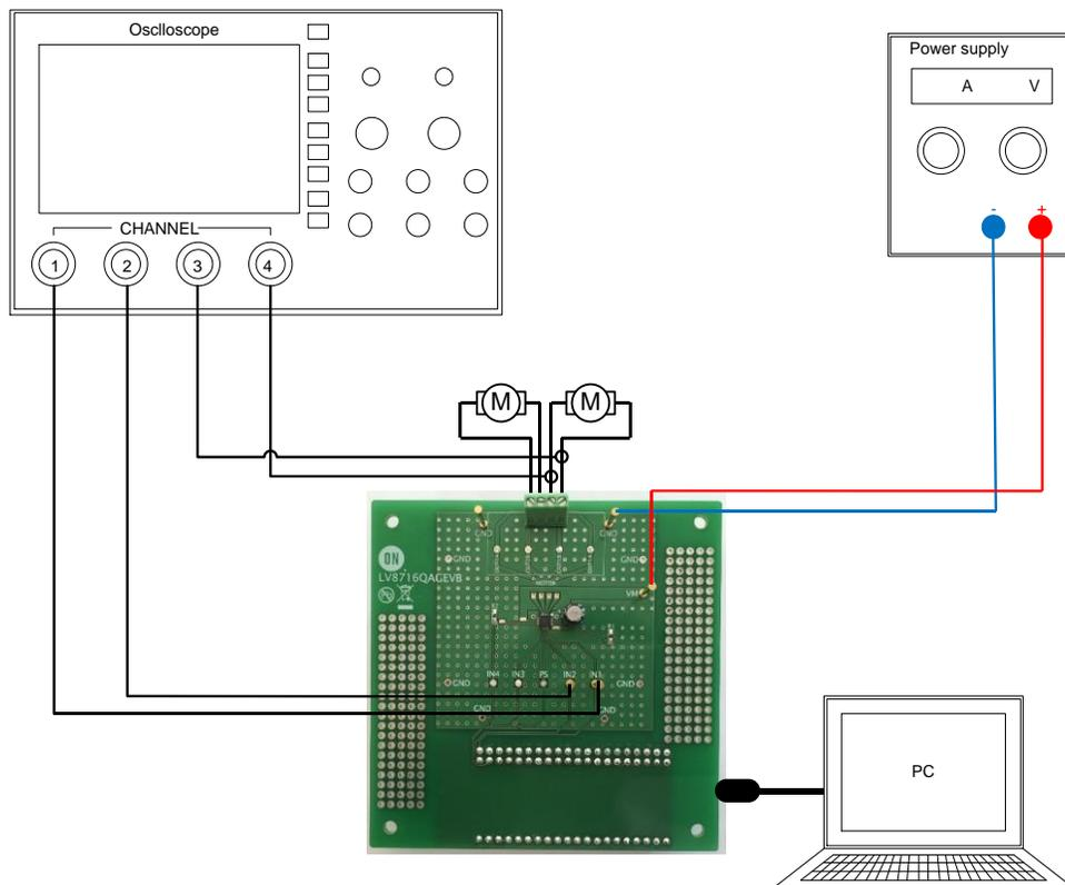
**Figure 36. Setup for a brush DC motor**
