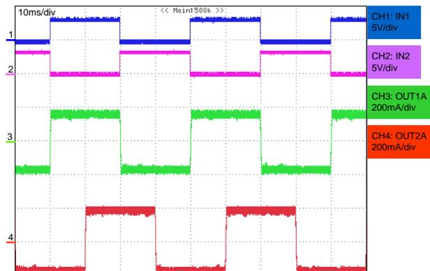
Figure 34. Full step setting waveform
