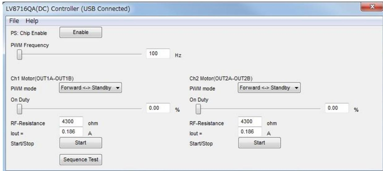
**Figure 26. GUI field description of DC controller window 2-1**
