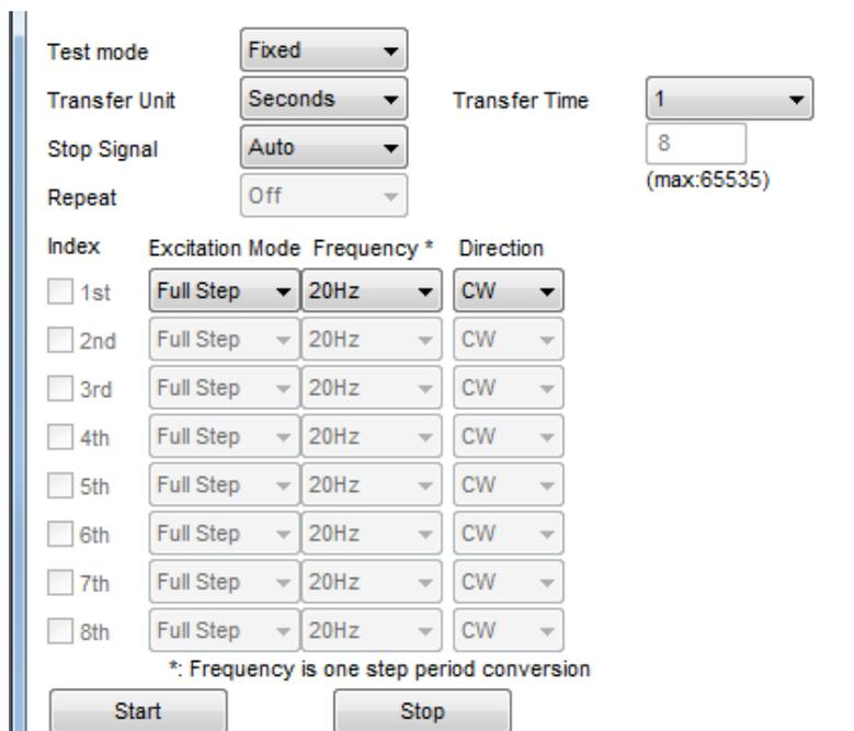
Figure 19. GUI field description of stepper controller window 1-2
