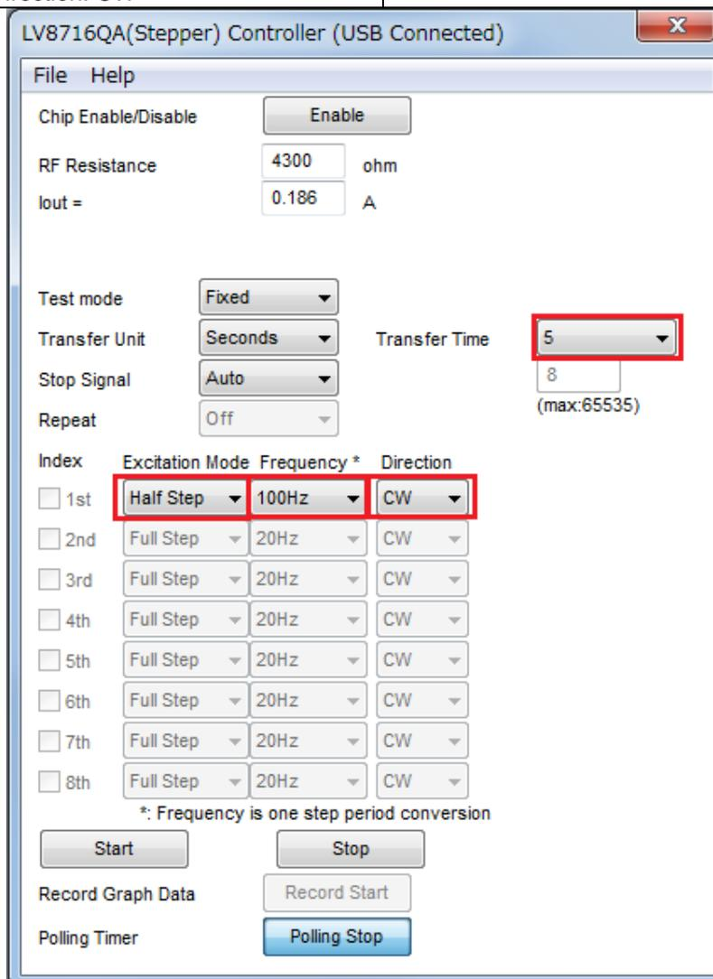
**Figure 33. Setting parameter of GUI for Stepper mode**
