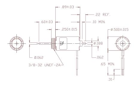
Solenoid shown energized and fully seated. Supplied with mounting bracket, hex nut and lockwasher (not shown). Spring kits are available (consult factory).
