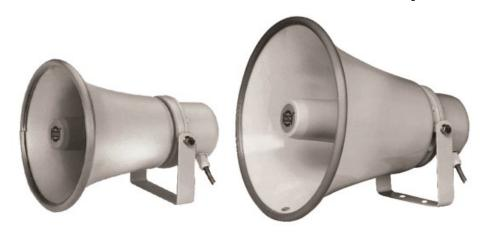
Rugged, weather resistant P.A. horn speakers manufactured with grey, epoxy coated aluminium. The horn has an integral 100V multi-tap transformer and power tapping switch which is easily selected from the rear of the unit using a screwdriver. Supplied with an adjustable U shaped mounting bracket.
