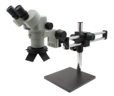
SPZ binocular stereo zoom microscopes offers the best in class zoom ratio with super sharp 3D images, wide field of view and long working distance which makes it an ideal choice for high throughput inspection stations and engineering and science labs.
