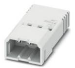
PCB connector, nominal current: 6 A, rated voltage (III/2): 160 V, number of positions: 4, pitch: 2.5 mm, connection method: Crimp connection, color: white
