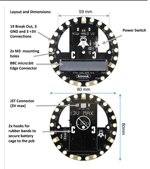
The Klip Halo board is 18mm thick (including BBC micro:bit and JST connector)
