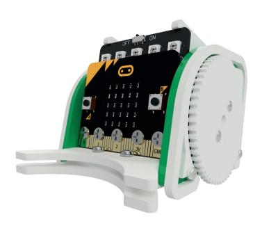
First, remove the lasercut panel from the front of the :MOVE mini.
