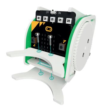
**NOTE:** The screws self tap into the holes on the lower panel.
