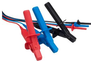
**10 kV lead set Cable insulation rating:** 12 kV d.c. (marked on cable) Cable type: flexible dual insulated silicon (inner insulation layer coloured white to highlight damage)
