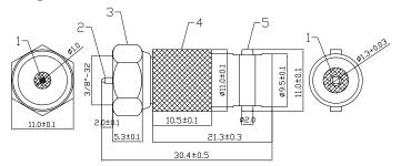
Item Designation Material POM 1 Dielectric 2 Pin Cu 3 Nut Cu 4 Middle Part Cu 5 **BNC Female Part** Zn
