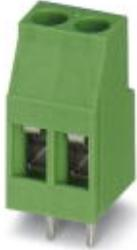
PCB terminal block, nominal current: 24 A, nom. voltage: 400 V, pitch: 5 mm, number of positions: 2, connection method: Screw connection with tension sleeve, mounting: Wave soldering, conductor/PCB connection direction: 0°, color: green. The article can be aligned to create different nos. of positions!
