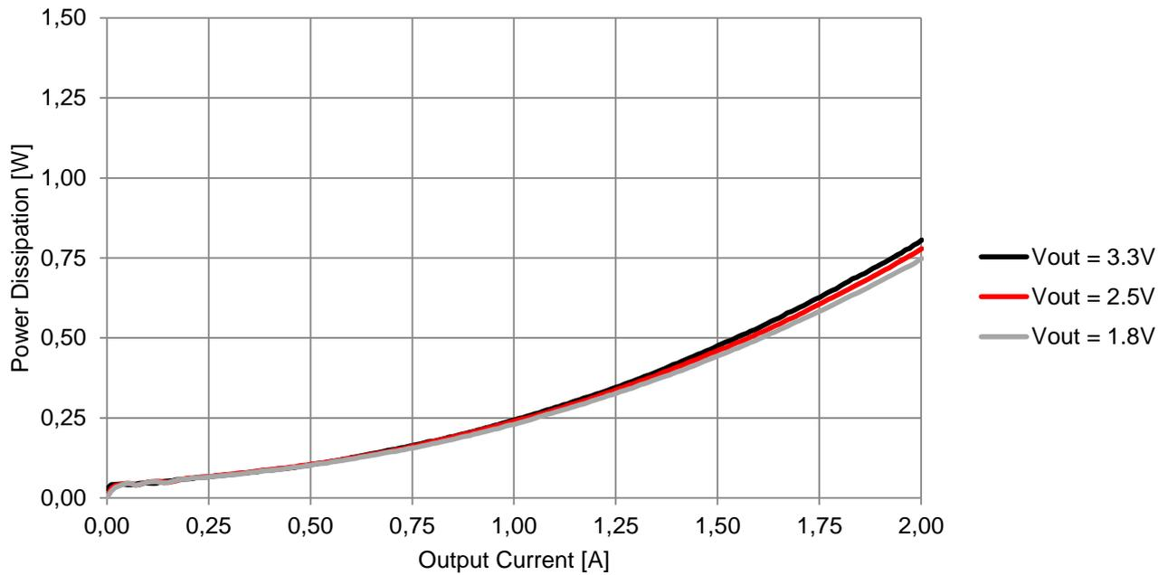
171021801  $V_{IN} = 5V$ ,  $T_A = 85^\circ C$
