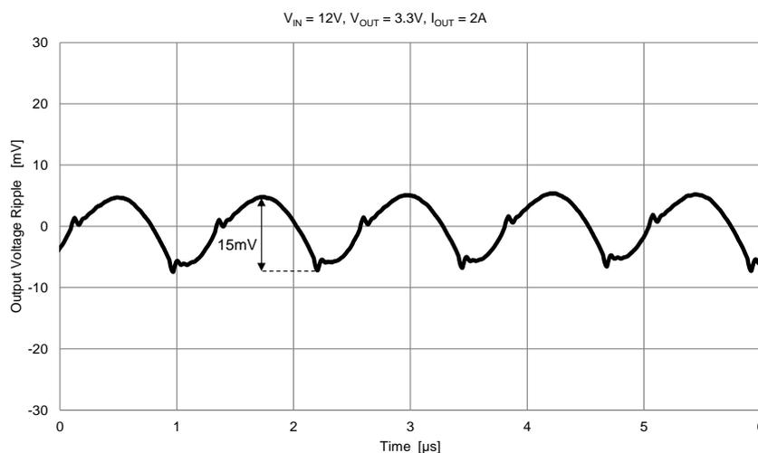
In case the application has more demanding requirements in terms of output voltage ripple, additional external capacitors should be used. The value of the external additional capacitance ( $C_{OUT,EXT}$ ) can be calculated using the following equation:
