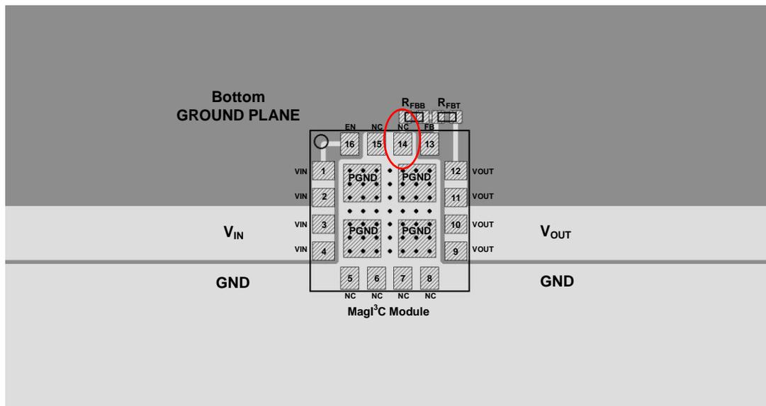
The ground connection of the lower resistor of the output voltage divider (R<sub>FBB</sub>) should be routed to the PGND pins of the device. If not properly handled, poor grounding can result in degraded load regulation or erratic output voltage ripple behavior.
