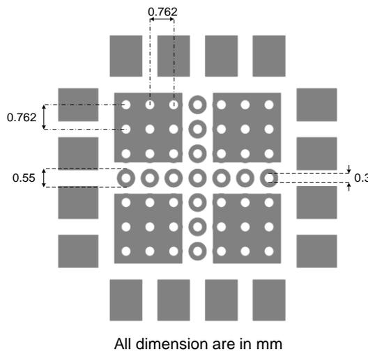
For best result, use a thermal via array as proposed in the picture above with drill of max 300µm, spaced 762µm apart. Ensure enough copper area is used for heat-sinking, to keep the junction temperature below 125°C. Connecting the NC pins (5,6,7,8) to the the GND layer helps dissipating the heat.
