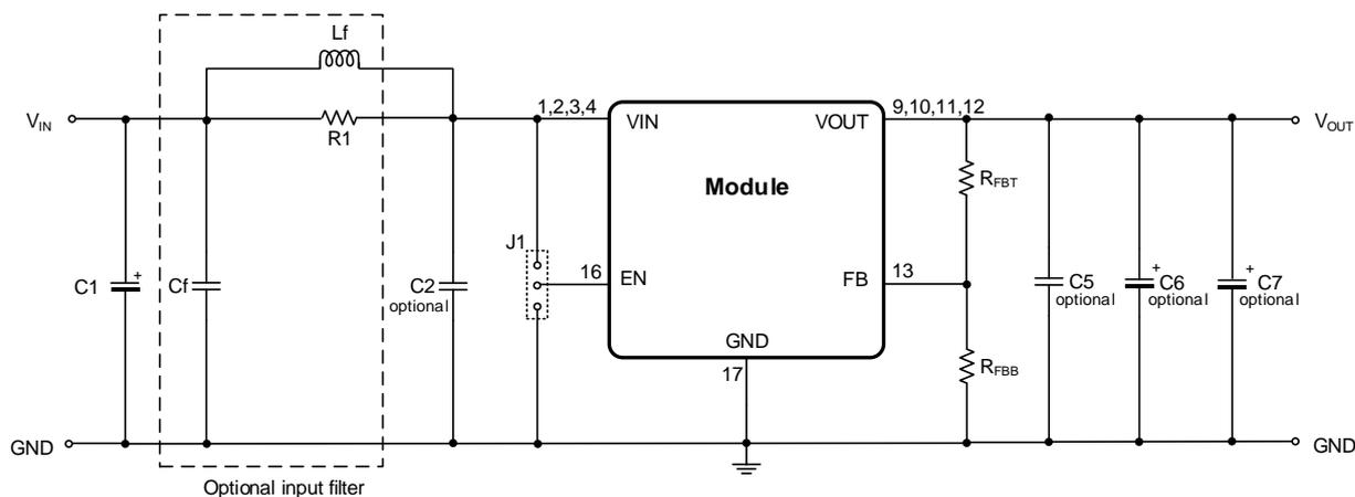
The 171021801 integrates both the input and output capacitors. Therefore, additional external input/output capacitors are normally not required.
