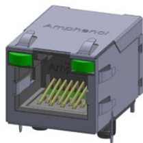
P/N RJE60-188-5XX1 SHOWN SINGLE PORT, 8 POSITIONS, WITH SHIELD AND LEDs CAT6A
