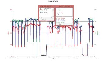
**RMS** - Trend current and voltage -- phase to neutral and phase to phase. Trend AC and DC simultaneously.
