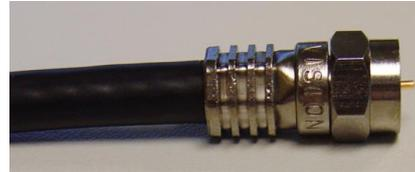
5. Using the chamfer inside the connector nut, push the connector ON the **wrong way** round to smooth the copper tape over the dielectric with a twisting action then remove and fit the correct way round.
