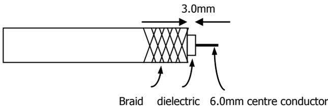
2. Carefully fold the exposed braid back over the sheath as evenly as possible
