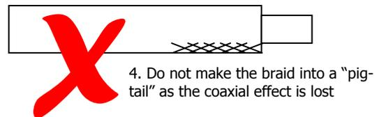
4. Do not make the braid into a "pig-tail" as the coaxial effect is lost
