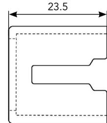
When pins are inserted into the panel mount receptacle half (SMS...R1) of the Quick Mating connector, an optional pin protection shroud can be installed.
