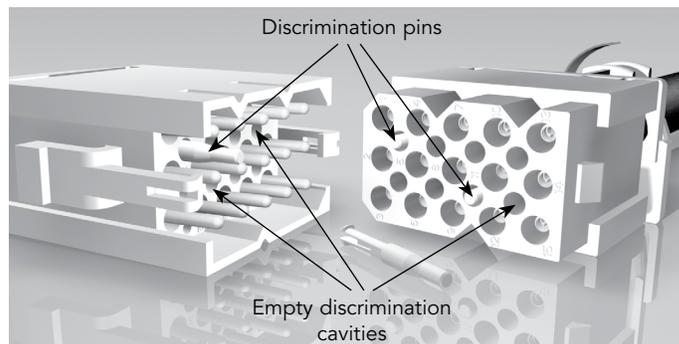
A pin, which can be inserted in the discrimination cavities of the SMS Quick mating cable and boardmount connectors. The discrimination cavities are in between of the contact cavities and offer the advantage that no contact cavities are lost due to discrimination.
