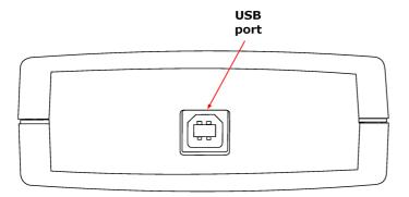
**USB port:** use the USB cable supplied to connect this to the PC that is running the Pico software. A PC with a USB 2.0 port is recommended for best performance.
