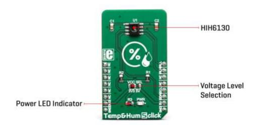
The HIH6130 features two ALARM outputs, which are used to indicate if the RH readings have exceeded, or fallen below a certain threshold, which can be programmed by the user, over the I2C. Besides the threshold values, the HIH6130 allows setting the polarity of the signal on these pins, as well as their driving topology (push-pull or open-
