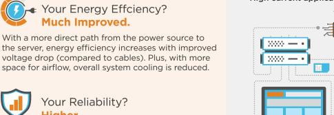
With limited cabled connections, the sliding power connector is also more reliable. There is no need for complex cable management or loose moving parts within the drawer. With a simple design, it is less prone to disconnection errors.
