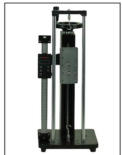
Stand with Optional Tensile Frame and Digital Scale
