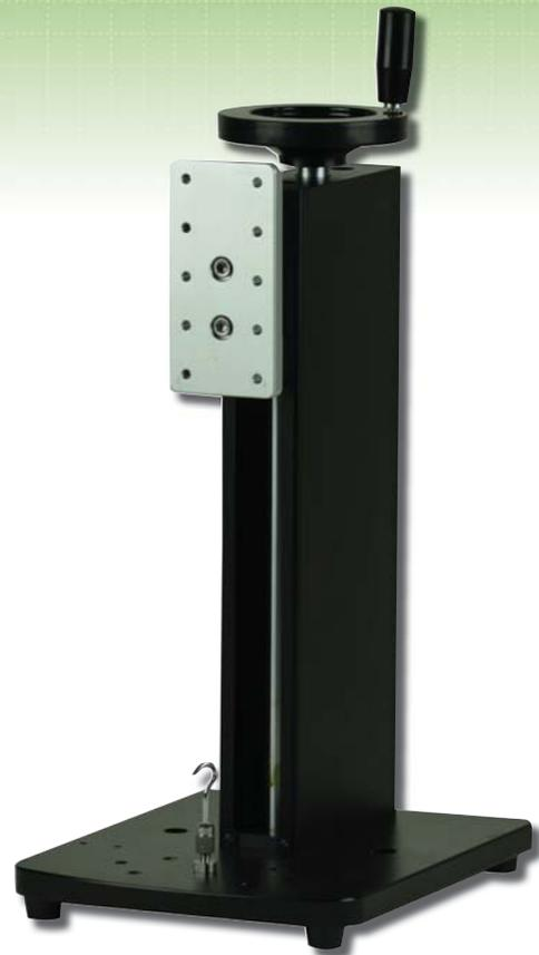
FGS-250W Manual Hand Wheel Operated Test Stand
