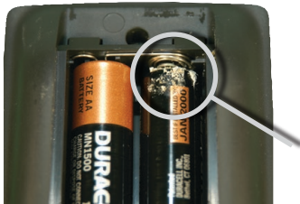
Corrosion you CAN see
