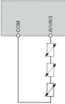
It is possible to connect either 1 or 3 sensors on terminals A1 or AI3
