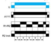
Before power-up Y1 should be permanently connected to A1.
