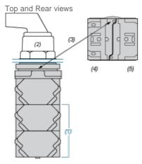
(1) It is possible to mount up to 3 levels of contacts blocks (maximum of 6 contacts blocks)
