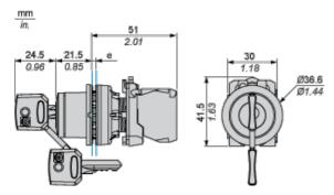
e: Clamping thickness: 1 to 6 mm / 0.04 to 0.24 in.
