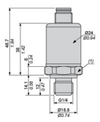
(1) SW24, tightening torque  $\leqslant$  24 N-m / 212 lb-in
