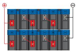
Figure 8. 3 Series x 2 Parallel connect modules. In this example, the system would provide 60 kW for 15 seconds at 168 V. Parallel cables (dashed lines) connecting modules in the middle are optional.
