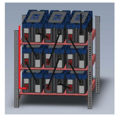
Figure 5. Nine series connected modules mounted in a 24" rack.
