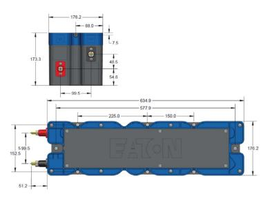
Figure 4. Dimensional drawing of module, all dimensions in mm.
