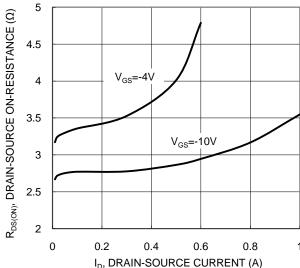
Figure 3. Typical On-Resistance vs. Drain Current and
