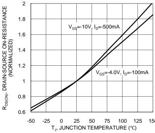
Figure 6. On-Resistance Variation with Junction Temperature
