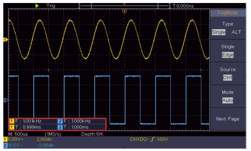
Figure 4-12 Automatic measurement
