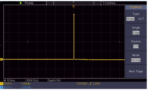
Figure 6-3 Capturing a Single Signal
