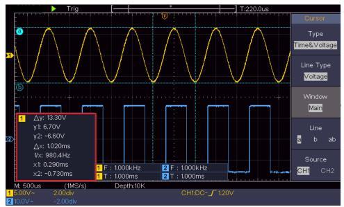
Figure 4-15 Time&Voltage Cursor Measurement
