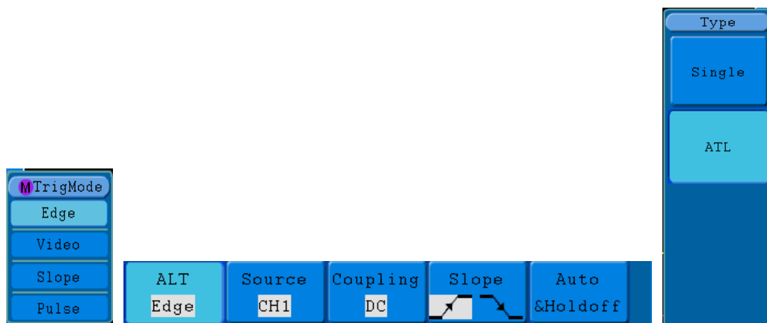
Figure 5-22 Alternate trigger (Trigger Type: Edge) Menu
