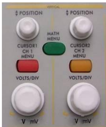
Fig. 4-9 Vertical Control Zone
