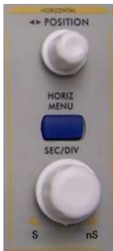
Fig. 4-10 Horizontal Control Zone
