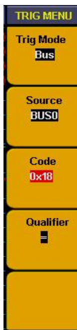
Fig.5-56: Bus trigger menu
