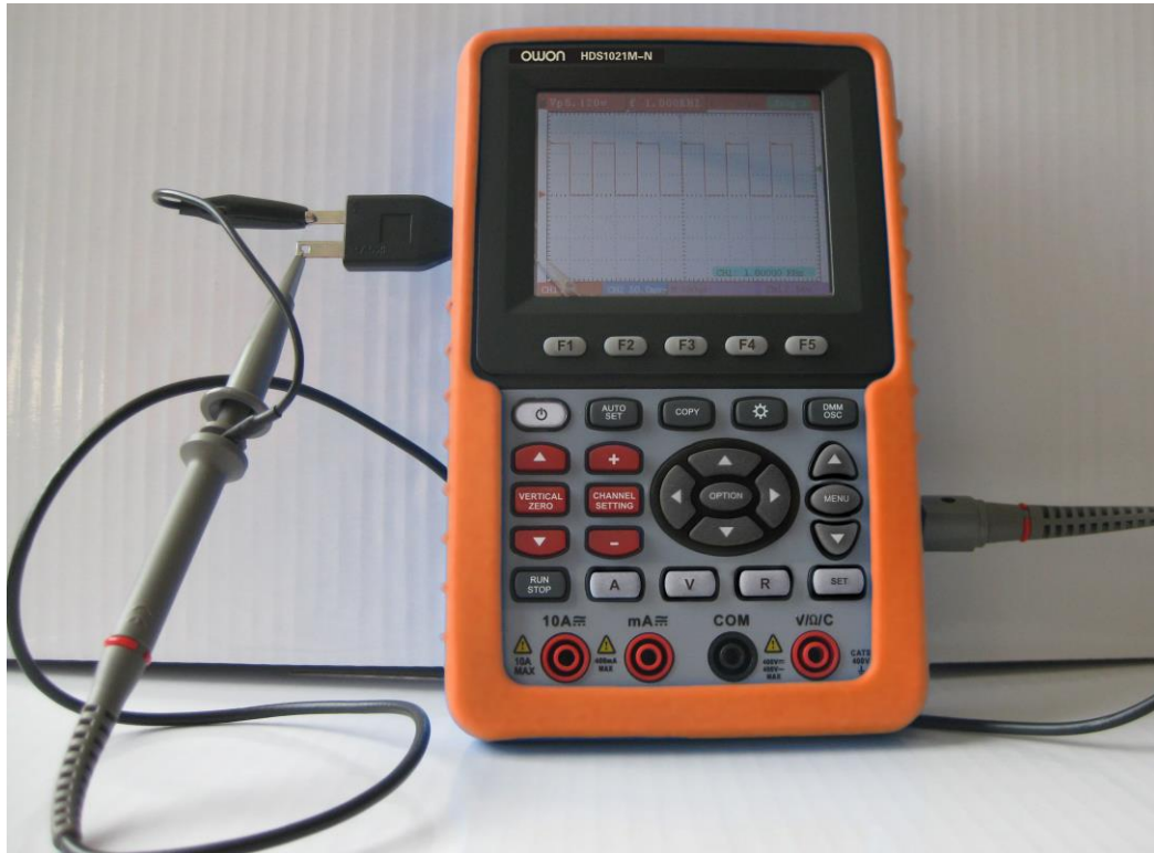
Fig.3. The connection of Square-wave test signal
