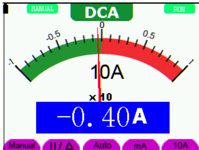
Figure 25: DC Current Measurement for 10A
