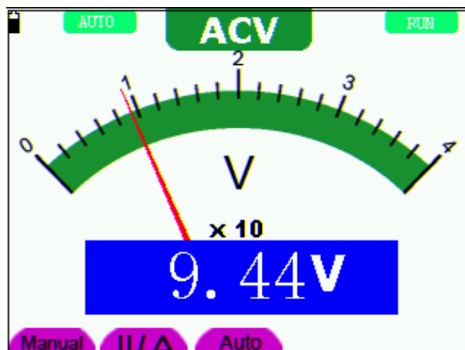
Figure 23: AC Voltage Measurement
