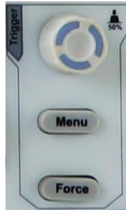
Figure 3-13 Trigger Control Zone
